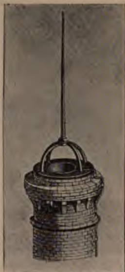
CHIMNEY TERMINALS OFTEN EM- PLOYED ABROAD.
